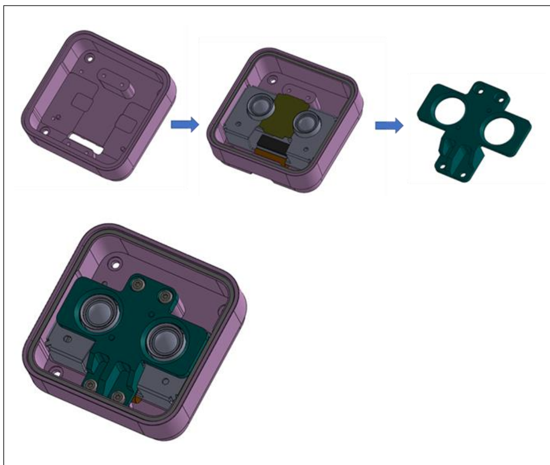
Figure 7-15. Stereo Depth Module Mid-Mounting – D401
